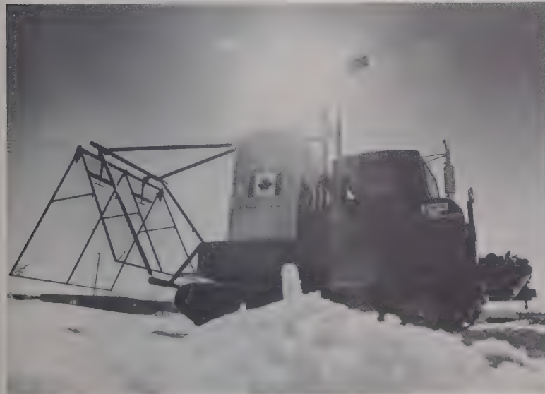
A snow tractor carries a large radar antenna that will be used to study the interiors of glaciers. The antenna, called the Radio Echo Sounding System, was developed by the Canadian government.
